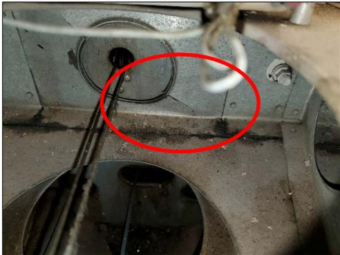
Pushing down on a horizontal stabilizer can cause internal damage that you won't be able to detect; the empennage is simply not built to withstand that kind of pressure. The pictures you see here show some bending and cracking of a stabilizer spar discovered during an inspection. It's impossible to tell exactly what event caused this, but it is the type of damage that can occur when downward pressure is applied to the horizontal stabilizers. Don't do it.
