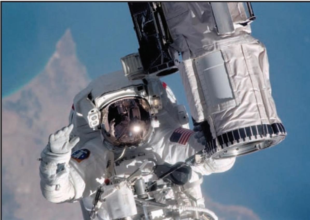
Astronaut holding on to an end effector attached to the robotic arm
