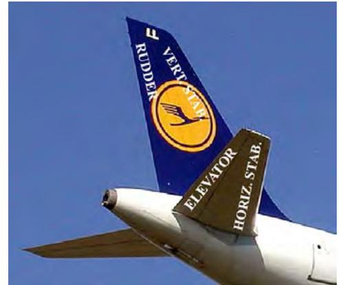
The thinner the atmosphere the slower the reaction of the airplane to its control surfaces. Airplanes flying at fast speeds in the lower atmosphere react more quickly to a change in the control surfaces than airplanes flying at extremely high altitudes at the same speed. That's because there are fewer air molecules to disturb. This becomes even more important when flying airplanes on planets with atmospheres that are less dense than Earth's atmosphere.
