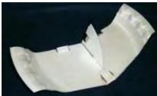
Rather than using paper to construct paper airplanes to use with this activity, you may wish students to construct foam plate gliders (FPGs) using foam plates, masking tape, and pennies. This will allow the ability to experiment with a rudder. The complete directions for constructing the gliders are available online at <http://www.modelaircraft.org/education/fpg-9.aspx> (AMA web page), courtesy of the Academy of Model
