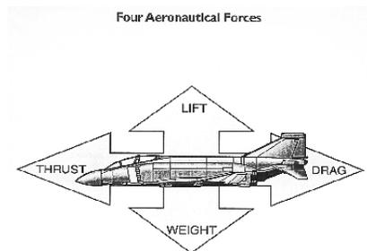
In aeronautics, there are four important forces. These four forces are called lift, weight, thrust and drag. Each force works in a specific direction. The magnitude of each force can vary from weak to strong. All of these four forces are hard at work when an airplane is in flight. They often work in opposite directions from each other, but together they make flight possible.
