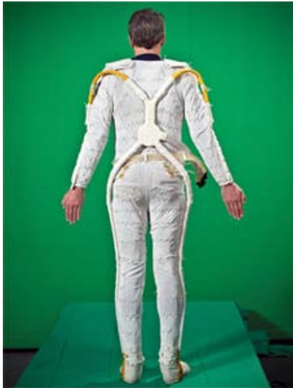
Liquid Cooling and Ventilation Garment Most long underwear keeps people warm. This underwear keeps spacewalkers cool.
