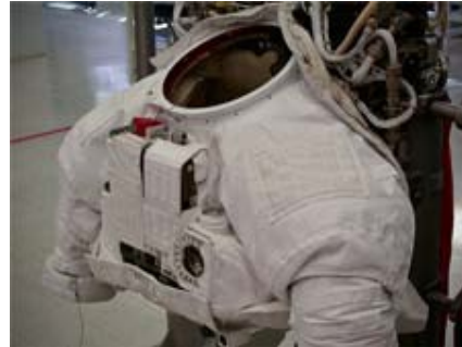
Upper Torso The top of the spacesuit includes the Hard Upper Torso (HUT) and the arm assembly.
