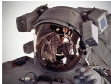
Helmet The bubble is covered by the Extravehicular Visor Assembly. The visor is coated with a thin layer of gold that filters out the sun's harmful rays. A TV camera and lights can be attached to the helmet.
