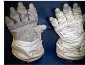
EVA Gloves Astronauts must be able to work with and pick up objects while wearing spacesuit gloves. EVA gloves are made to protect astronauts from the space environment. They are also made so spacewalkers can move their fingers as easily as possible. The fingers are the part of the body that gets coldest in space. These gloves have heaters in the fingertips. A piece called a bearing connects the glove to the sleeve. The bearing allows the wrist to turn.
