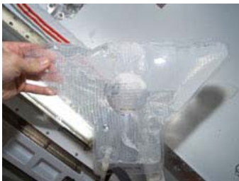
In-Suit Drink Bag A plastic, water-filled pouch attaches to the inside of the Hard Upper Torso using Velcro. A plastic tube with a valve sticks out of the bag. The tube and valve can be adjusted to be near the astronaut's mouth. Biting the valve opens the tube so the spacewalker can take a drink. Releasing the bite closes the valve again.
