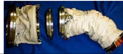
Arms Spacewalkers do not wear custom-made suits. Different sizes of arm assembly parts are available.
