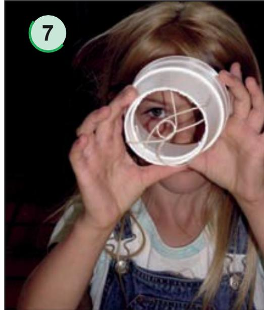
*You have now created an "Effector" and it will pick up a small object like a pencil. Have someone hold the pencil upright. Open the end effector so that the strings are not crossing each other. Slip the end effector over the pencil so that it extends down the center and not through any of the loops. Rotate the outer cup until the strings grasp the pencil. You should now be able to pick up the pencil.*
