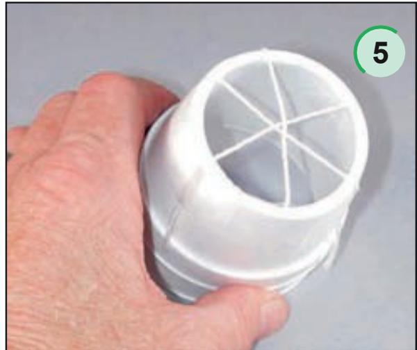
*While holding the rim of the inner cup, rotate the outer cup until the three strings cross each other. The strings will have some slack. Pull the end of the strings on the outside until they are straight and intersect in the middle. Now press the tape on the outside to hold the strings.*
