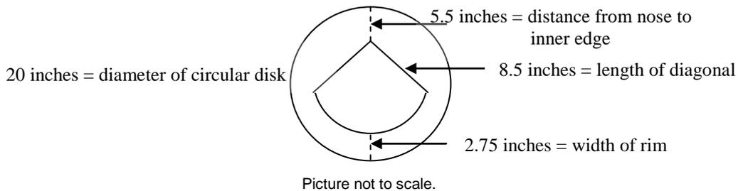
You can make 4 Geobats from a 4' x 4' piece of Dow blue foam (or similar foam insulation board).
