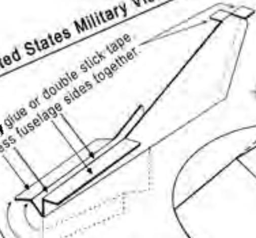
After applying adhesive to fuselage, mount to underside of wing.
