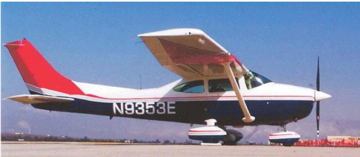
This is a picture of a Civil Air Patrol Cessna. It clearly shows the shape of a wing. Notice how it is curved on the top. This is what gives the wing most of its lifting capability.
