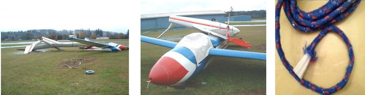
This damage was the result of only a 45 mph wind gust when improper ropes were used.
