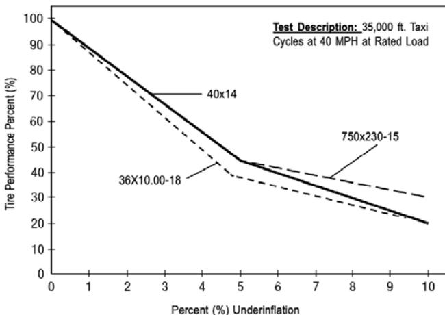
Fig 1: Fatigue Due to Under-inflation
