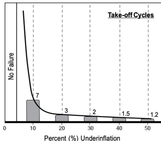
Fig 2: Cycles to Failure
