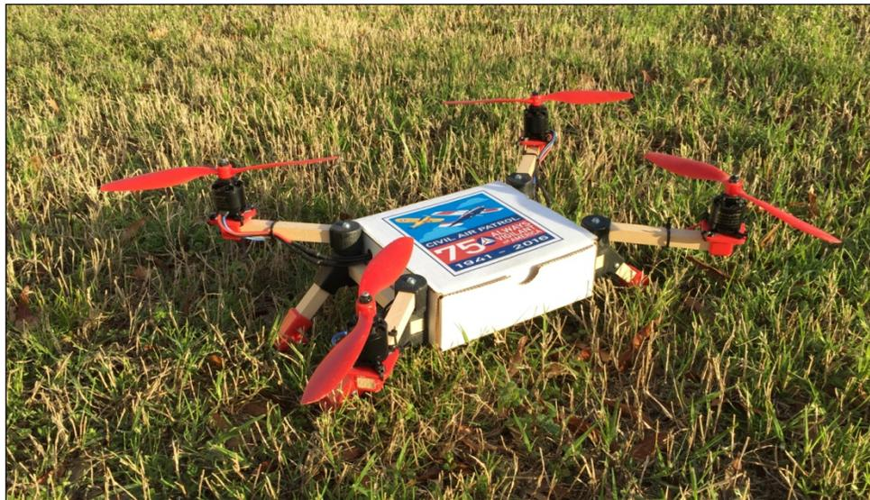
While some are equipped with rotor guards, many are not which increases the risk of unintentionally hitting something with a rotor.
