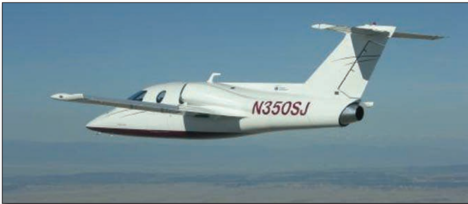
3.5 This is a Sport Jet II. This aircraft brings corporate jet performance to the world of home-built aviation. At 380 knots, it easily cruises at 28,000 feet for 900 miles. It does not require two pilots and will carry four in a luxury cabin. The cost is less than a million dollars to build and fly. (Image is courtesy of Excel Jet)
