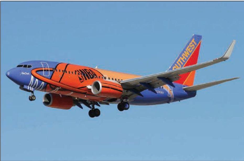
3.7 Throughout the flight profile, there are dramatic changes in pressure, from 29.92 inches at sea level to 5.3 inches at 40,000 feet, and back again. (Image is courtesy of Ben Wang and Airlines.net)
