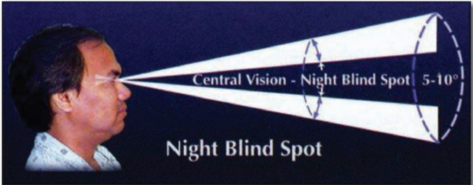
3.16 The night blind spot is approximately 5-10° in the central vision. (FAA Illustration)
