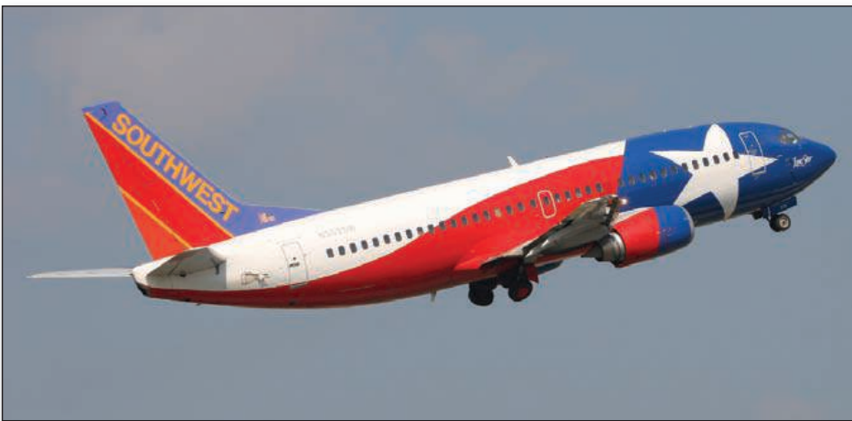
2.11 On hot days at high altitude airports, airplanes don't get off the ground as quickly because the air density is less. Although the actual airport altitude may be 5,431 feet, the airplane is performing like it would at 8,000 feet or higher. This is known as high density altitude. (Photo by Adam Wright)
