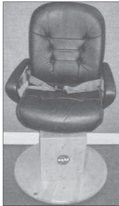
C-16 – This is the NASA version of the Barany chair. Note the round base, the varnished finish, and the seat belt.
