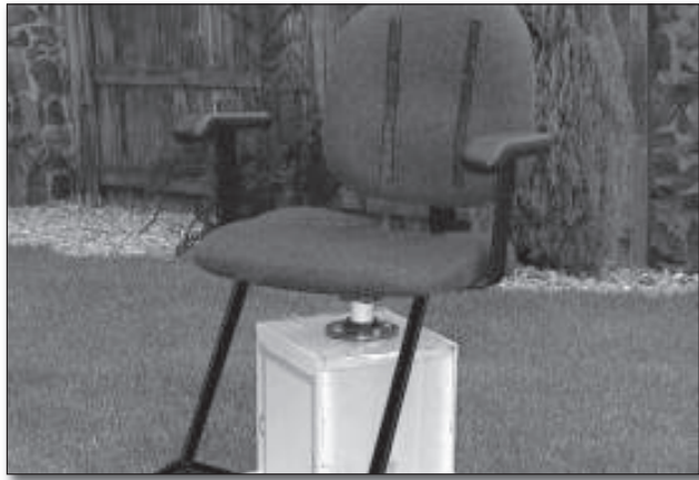
C-1 – This is a completed, homebuilt Barany Chair: It is essentially an office chair that is mounted on a milk box. The chair rotates on an automotive axle housing and when properly installed, the chair will rotate quietly, and with very little friction. The pilot sits blindfolded holding a joystick. When the chair is slowly rotated, the pilot moves the joystick to show the direction in which he/she is rotating. As the chair is allowed to slowly come to a stop, the inner ear mechanism will tell the pilot he/she is still moving, but in the opposite direction. The text gives the construction details and explains how the disorientation occurs. This is not a toy and the presenter should not allow it to be rotated at high speed.
