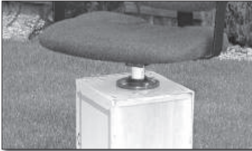
C-20 – The rigid coupling spacer is shown between the chair and the axle bearing.
