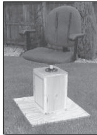
3.3 A homemade Barany chair. The Conference Guide that follows shows how to make this educational device. Using automotive rear axle housing, a milk box, and an used office chair. Once a footrest is installed, pilots sit comfortably, blindfolded, and are slowly rotated. The experience is fun, yet sobering. It’s an excellent way to gently show the effects of vertigo and disorientation.
