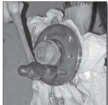
C-11 – The studs are first removed from the axle bearing assembly.
