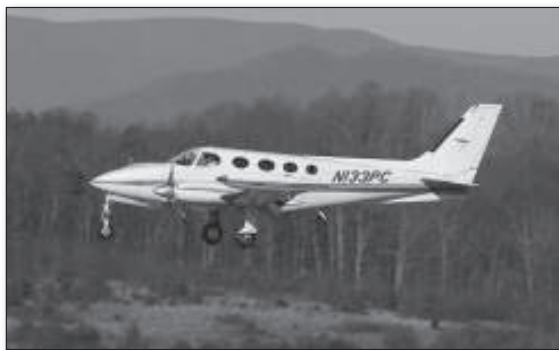
2.3 On days when it is hot and humid, pilots experience the effects of density altitude as the airplane climbs out during takeoff. (Image by Adam Wright)
