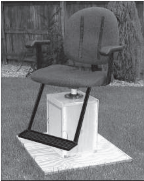
C-22 – Using a little “ingenuity,” build a footrest to keep the legs from swinging during slow rotation.
