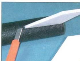
The fin is now placed on the pipe foam covering the seam. This seam acts as a positioning guide.
