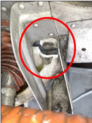
symptoms seriously! If you detect these, abort the mission and get the aircraft checked by an A&P. It may seem like a small controllable issue at the moment but you don't want to take the chance of the situation worsening. There is nothing "normal" about an aircraft that doesn't handle correctly. You may very well be the person that is first to discover a crack, and the person who prevents a mishap.
