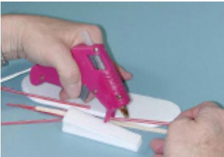
Step 3 – Using the template as a guide, glue the four plastic coffee sticks into place along the fuselage.
