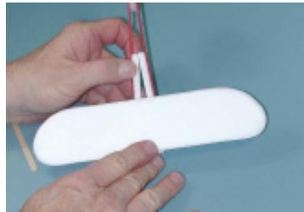
Step 7 – The horizontal stabilizer is mounted at the back near the rudder. Note that it is on the bottom of the fuselage coffee sticks. Check the illustration on how this is positioned.
