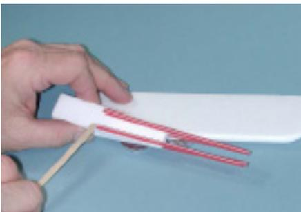
Step 4 – Glue the rudder to the ends of the four fuselage stirring sticks.
