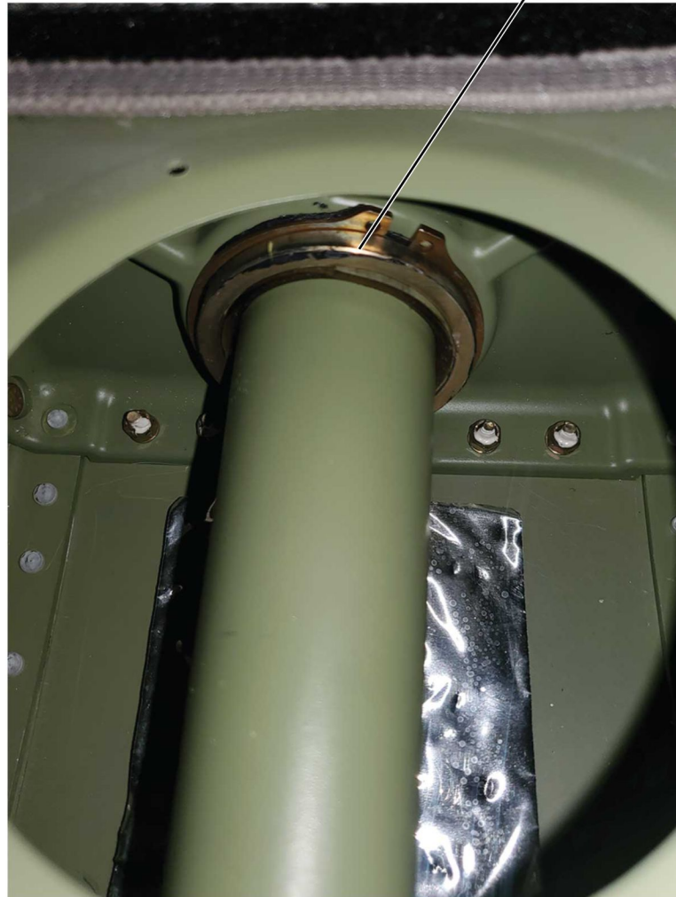
Good Bushing (View Looking Outboard at Left Gear Bushing)
