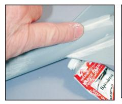
White glue can be used to make a nice, rounded fillet between the fins and body. Apply the glue and run your index finger along the length of the joint. The finger provides a nearly perfect form for the fillet. Glue may be easily removed from fingers with water.
