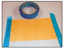
Masking tape can be used to hold sandpaper to a flat surface. This makes a solid base for sanding edges and flat surfaces.
