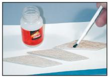
It is highly recommended that the builder use a sanding sealer on the balsa. This seals the surface and makes a more professional looking paint finish.
