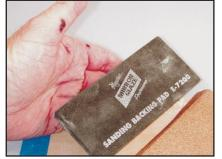
The builder can also use a sanding block. The paper is wrapped around a block for sanding the balsa pieces. This creates a flat surface when sanded.
