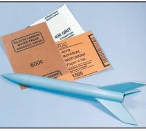
Once the rocket is completely assembled and all balsa components sealed, it is ready to be painted. After spraying one or two coats of primer, carefully sand the surface with a finer grade of paper. It is recommended that the builder let the rocket set overnight so the primer has a chance to cure. It is also recommended that very fine sandpaper be used for the final primer coat sanding step.
