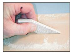
The fins can be held together, and the surfaces sanded. This makes all of the fins uniform.
